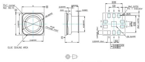
Dimensions are in millimeter unless otherwise specified General Tolerance is +/-0.10mm unless otherwise specified
